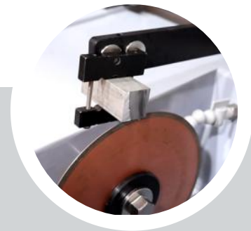
Five kinds of ( Accessories) fixtures enables the processed work piece to be sectioned at the optimal angle
